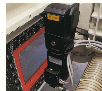
Dust collector system with PU spiral hose directly connected into the closed cutting area. Dust emissions far below the requirements of the safety and health dept.
