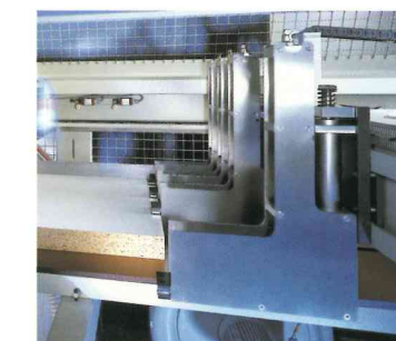
Floating grippers with rubber pads.
