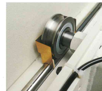
Material pusher table with two hardened and polished guide ways, hardened guide rollers, concave, in full contact with guide bars.
