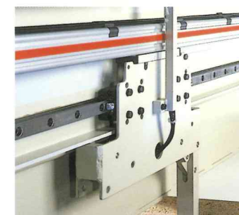
Fully automatic side aligner with pneumatically controlled pressing finger.
