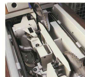
Saw carriage with two hardened and polished guide ways moving on Star guide bearing assemblies.
